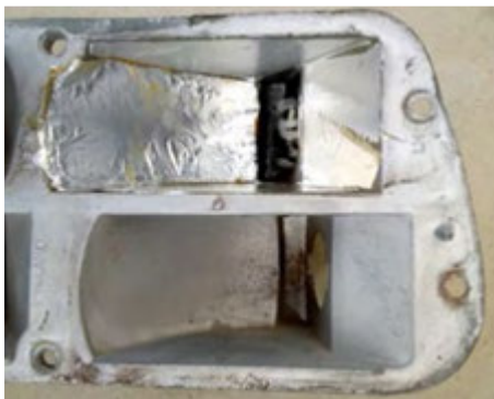
Left: Aluminium foil glued inside housing Below: Extra connection to the earth tab
