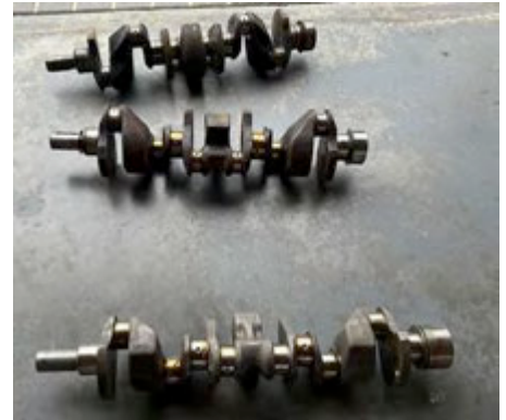
3 cross drilled crank shafts. The bottom one is Vanguard 6. Ex race engine with 7 bolt Flywheel to Crankshaft. all 3 in exceptionally good condition
