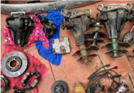
Diffs 3.4 3.7 4.1. 4.1 has chipped tool on crown wheel
